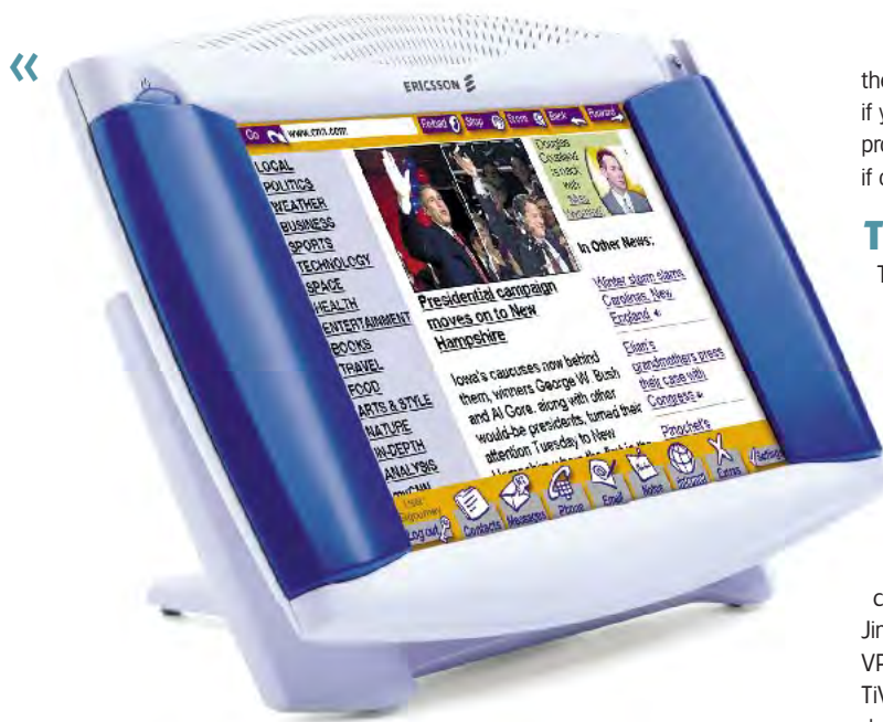
The Ericsson Screenphone, a Linux-based Internet Appliance.
