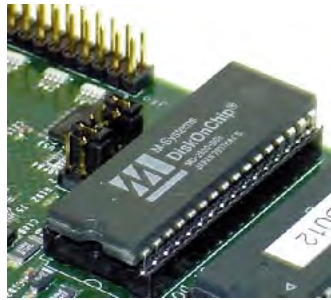
DiskOnChip is an alternative storage system to FLASH for embedded devices.
