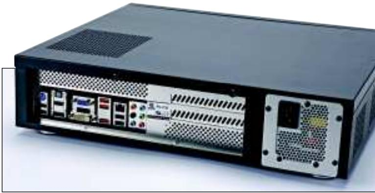
› The case we've chosen will only fit a micro-ATX board. This is a form factor several revisions smaller than standard ATX.
