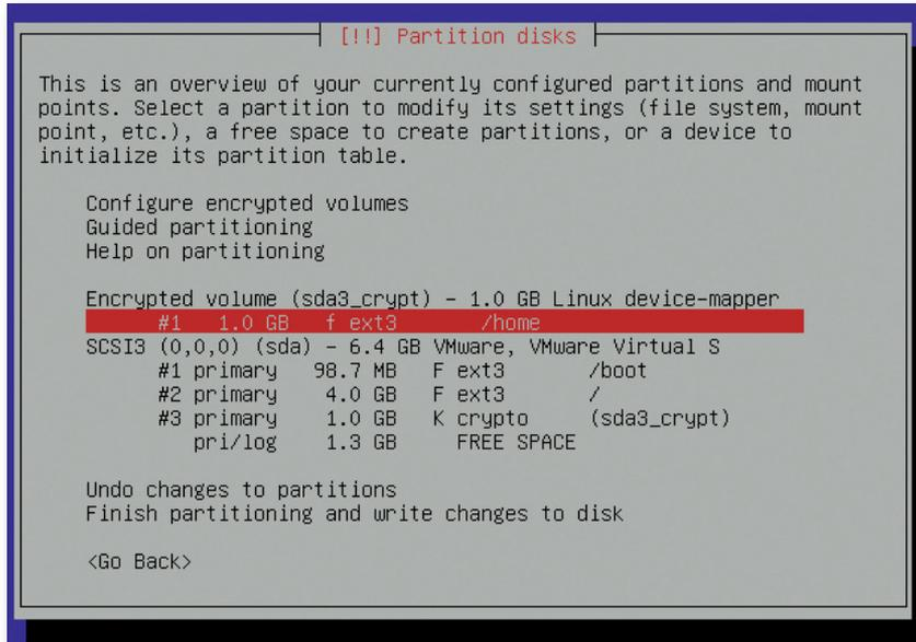
▶ Manual configuration of encrypted partitions needs care. Here, `/home` is mounted from the encrypted partition `sda3_crypt`.
