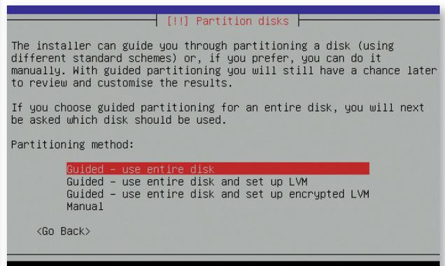
› Installing from the Ubuntu 8.10 'Alternate' CD offers an easy way to set up an encrypted filesystem.
