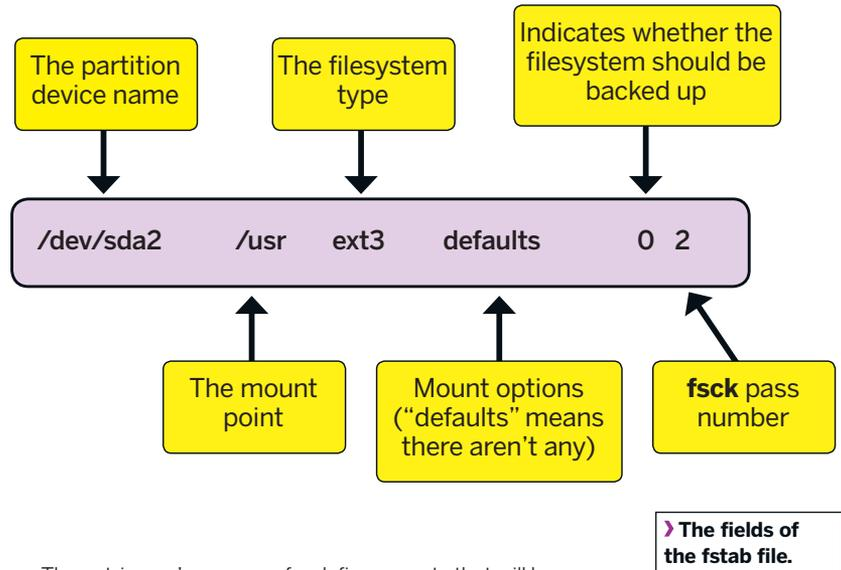
The entries we've seen so far define mounts that will be performed at boot time, in response to a `mount` – a command buried somewhere in a boot script. The diagram below shows an entry for a removable device such as a CD. This line is not there to define a boot-time mount, but to make mounting of removable media easier. For one thing, it means you can mount a CD just by typing a command such as
