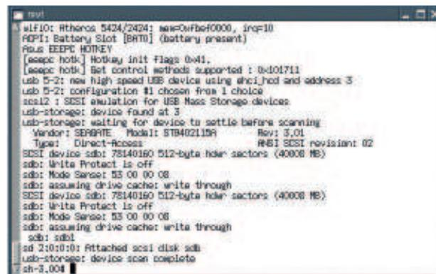
» Using the `dmesg` command we can identify the device name of an external drive so that we can mount it.
